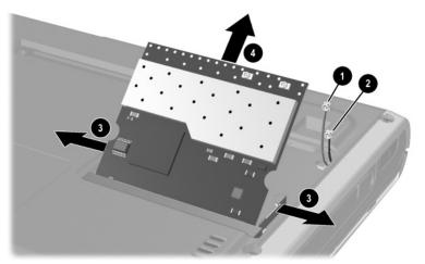
Removing a Mini PCI Communications Board
